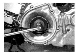
• Remove the generator rotor cover and exhaust cover stay.
